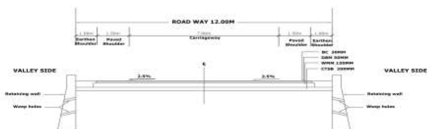
Fig - 2.12 (new) Typical Cross Section (Hilly Terrain) 2-lane carriageway (With Paved Shoulder) (With Retaining Wall on both Side)
